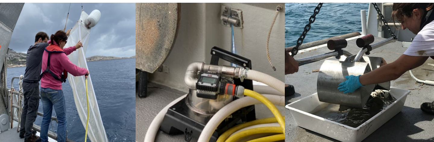
Three different types of sampling equipment were used on this research cruise including (from L-R), a manta trawl, the new ferrybox microlitter sampler, and a sediment corer (Image Credit: Francois Galgani).
