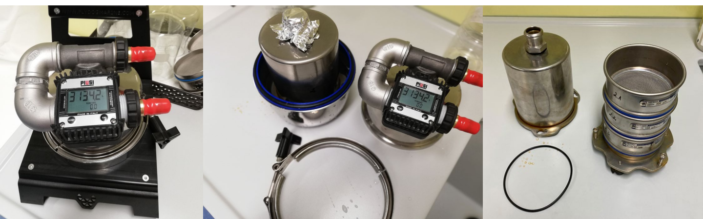
Pictured (from L-R) is the completed JPI Oceans ANDROMEDA microlitter sampling device, the device with the outer container opened, and the inner container with three ascending sieves (Image Credit: Urmas Lips).
